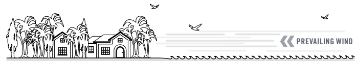
REGION A - N3 (W41) REGION B - N4 (W50) AND REGION C - C3 (W60) THE FIRST ROW OF BUILDINGS ADJACENT TO THE SEA FRONT
