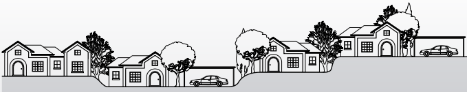
REGION A - N2 (W33), REGION B - N3 (W41) AND REGION C - C2 (W50) STRUCTURES ON UNDULATING TERRAIN IN SUBURBIA
